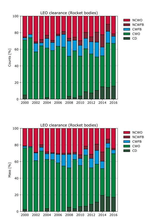
Figure 6.3: Relative share in terms of number (top) and mass (bottom) of disposal behaviour classes for Rocket Bodies in LEO.
