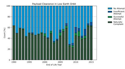
(a) Relative clearance of  $\ensuremath{\text{LEO}_{\text{IADC}}}$  by payloads.
