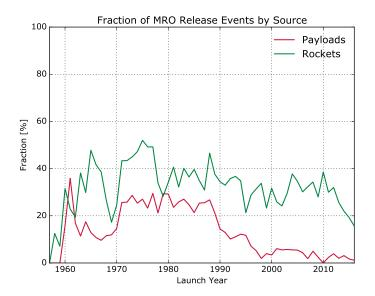
Figure 4.2: Fraction of mission related objects releases per year w.r.t. the total amount of payloads and rocket bodies injected into the space environment during that year.
