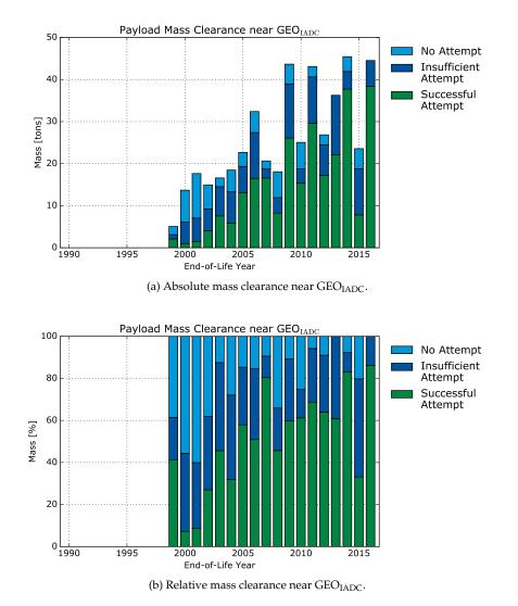
Figure 6.14: Mass trend of adherence to the disposal guideline in  $GEO_{IADC}$ .
