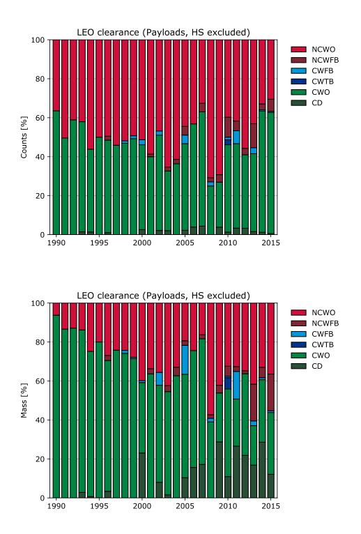
Figure 6.2: Relative share in terms of number (top) and mass (bottom) of disposal behaviour classes for payloads in LEO, excluding objects associated with human spaceflight.
