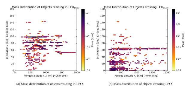
Figure 3.4: Distribution of mass in LEO as a function of inclination and perigee altitude.
