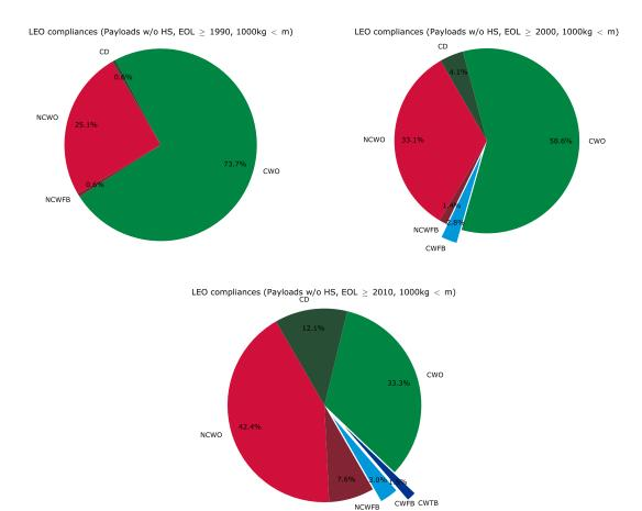
Figure 6.11: Breakdown per decade (1990 top left, 2000 top right, 2010 bottom) of observed behavioural classes for payloads with a mass above 1000.0 kg.
